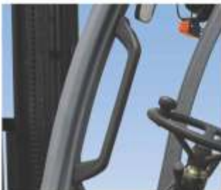
Large operator hand assisted access grip
