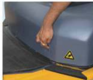
Lever for smooth opening of engine hood
