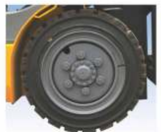
28 x 9 x 15 front tyres for better road grip and higher stability
