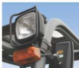
Protective light guards prevents damage
